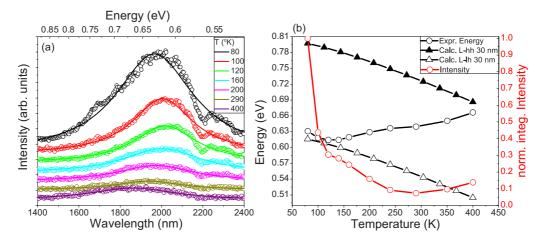
FIG. 3. (a) Photoluminescence spectra of Ge/In<sub>0.24</sub>Ga<sub>0.76</sub>As (sample E) under  $\varepsilon = 1.6\%$  biaxial tensile strain depending on temperature; (b) experimental (circles) and calculated (triangles) peak energy (black line) and normalized integrated intensity (red line) versus temperature.
