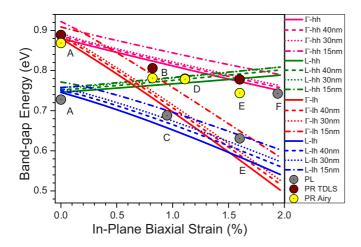
FIG. 8. Theoretical band-gap-strain dependence for Ge calculated using a  $30 \times 30$   $\mathbf{k} \cdot \mathbf{p}$  model taking into account quantization-induced band-gap enhancement at decreased  $\varepsilon$ -Ge layer thicknesses for 40-, 30-, and 15-nm quantum wells. Experimental peaks given by PL and PR data are shown as circles over theoretically predicted transitions from  $\Gamma$  and L valley to light (lh) and heavy (hh) holes.
