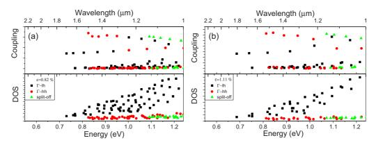
FIG. 11.  $\mathbf{k} \cdot \mathbf{p}$  calculations of electron-hole wave-function coupling and density of states (DOS) for subband transition energies in (a) 40-nm Ge quantum well with  $\varepsilon = 0.82\%$  biaxial tensile strain; (b) 30-nm Ge quantum well with  $\varepsilon = 1.11\%$  biaxial tensile strain.
