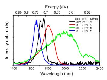
FIG. 5. PL spectra at different biaxial tensile strain (samples A, C, E, F) at 80 K.
