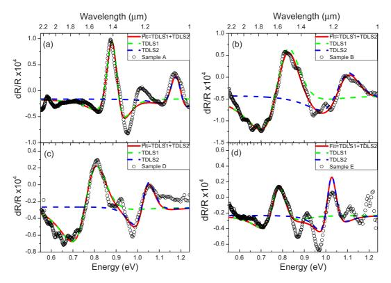
FIG. 6. Photoreflectance spectrum of Ge under  $\varepsilon$ : (a) sample A, 0%; (b) sample B, 0.82%; (c) sample D, 1.11%; (d) sample E, 1.6% biaxial tensile strain at 80 K, fitted with two TDLS functions. Open circles correspond to the experimental data, red lines are the fit including two TDLSs, depicted in green and blue, respectively.
