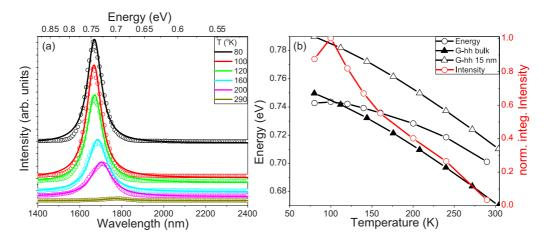
FIG. 4. (a) Photoluminescence spectra of InGaAs/Ge/In<sub>0.29</sub>Ga<sub>0.71</sub>As/GaAs (sample F) under  $\varepsilon = 1.94\%$  biaxial tensile strain depending on temperature; (b) experimental (circles) and calculated (triangles) peak energy (black line) and normalized integrated intensity (red line) versus temperature.
