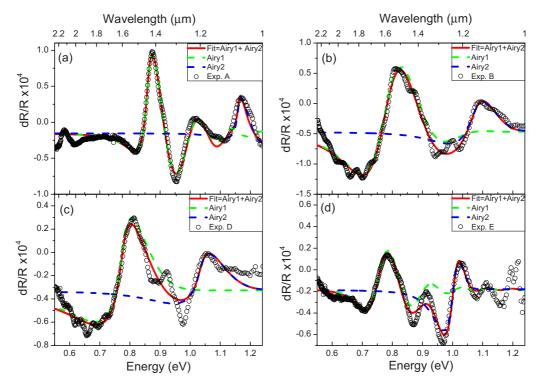
FIG. 7. Photoreflectance spectrum of Ge under  $\varepsilon$ : (a) 0%, (b) 0.82%, (c) 1.11%, (d) 1.6% biaxial tensile strain at 80 K, fitted with two Airy functions. Dotted lines correspond to the experimental data, red lines are the fit including two Airy functions, depicted in green and blue, respectively.
