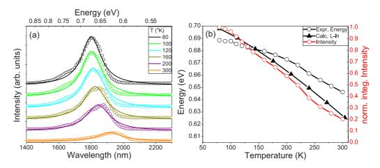
FIG. 2. (a) Photoluminescence spectra of  $GaAs/Ge/In_{0.16}Ga_{0.84}As/GaAs$  (sample C) under  $\varepsilon = 0.95\%$  biaxial tensile strain depending on temperature; (b) experimental (circles) and calculated (triangles) peak energy (black line) and normalized integrated intensity (red line) versus temperature.
