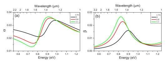
FIG. 12. Calculated (a)  $\alpha$  and (b)  $\beta$  Seraphin-Bottka coefficients in Ge at 80 K and at 0%, 0.8%, and 1.1% biaxial tensile strain.
