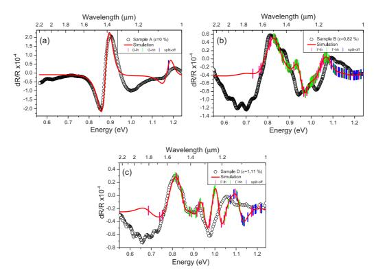
FIG. 9. Full photoreflectance spectra simulation on the top of experimental data for (a) unstrained sample; (b)  $\varepsilon = 0.82\%$  model over sample D spectra; (c)  $\varepsilon = 1.11\%$  model over sample E spectra.  $\Gamma$ -lh,  $\Gamma$ -hh, and split-off subband transition energies are depicted as vertical dashes.
