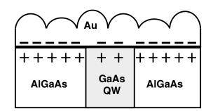
FIG. 3. A schematic diagram of the geometry used for the theoretical simulation. The + symbols represent the positive interface state charge, which is larger on the metal-Al<sub>0.3</sub>Ga<sub>0.7</sub>As interface than on the metal-QW interface. The - symbols represent the image charge in the metal film.
